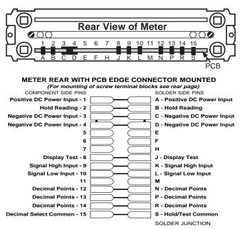
**Pins 1 & A - Positive DC Power Input:** These pins are internally connected together. The positive end of the DC power is connected to these pins. The standard BN-351 meter is designed to be powered from a 24VDC power supply. Optional 5V, 12V, or 15VDC powered models are also available. Before using the meter, make sure that the appropriate power is being applied. The BN-351 meter generates a ±5V supply internally that is isolated from the applied DC power.
