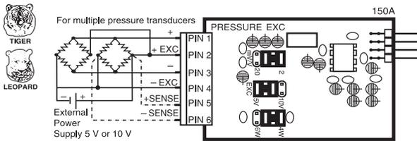
**IS05:** Pressure/Load Cell 20/2mV/V, 5/10V Exc 4-wire
