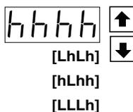
When there are more than two display selections they are shown in brackets below the first display and are also selectable by pressing and releasing the **↑** or **↓** buttons.
