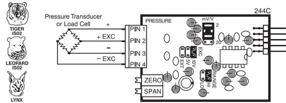
**IS06:** Pressure/Load Cell Ext Exc., 20/2mV/V, 4-wire
