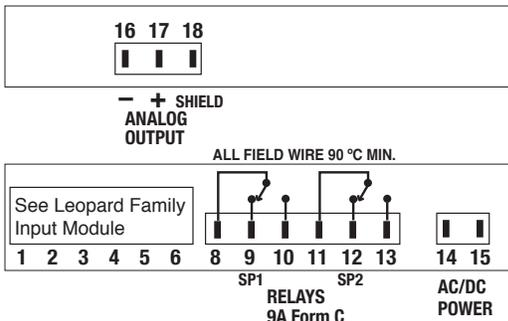
Auto-sensing AC/DC power supply. For voltages between 85-265 V AC / 95-300 V DC (PS1) or 15-48 V AC / 10-72 V DC (PS2).
