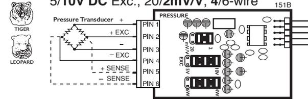
**IS04:** Pressure/Load Cell Ext Exc., 20/2mV/V, 4/6-wire
