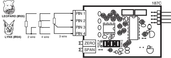
**IS01:** Strain Gage 5/10V DC Exc., 20/2mV/V, 4/6-wire
