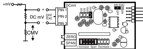
Can be used to measure single-ended or differential inputs.
