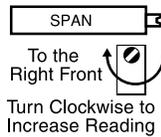
The 15 turn SPAN pot is always on the right side (as viewed from the front of the meter). Typical adjustment is 100% of the input signal range.
