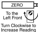
The ZERO pot is always to the left of the SPAN pot (as viewed from the front of the meter). Typically it enables the displayed reading to be offset  $\pm 100$  counts.
