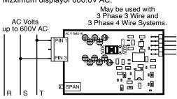
The unique differential input allows safe phase to phase AC true RMS line voltage measurements up to 600V AC.
