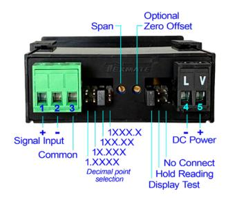
For the non-isolated 5VDC power supply option, DC Power Pin 4 (-) is electrically connected to Common Pin 3. For the isolated power supply options, the two pins are not electrically connected (isolated).
